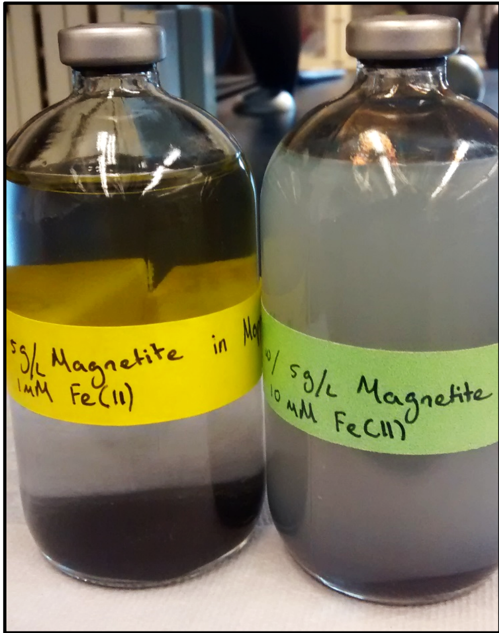
Figure 11. Images of 50 \mu\text{M} TCE reactors with low Fe(II) (Left reactor) and precipitated \text{Fe}(\text{OH})_2(\text{s}) (Right reactor) with 5 g/L magnetite in 10 mM MOPs buffer at pH 8.0.
